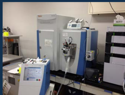
Orbitrap フーリエ変換型MS (Q-Exactive ThermoFisher)
